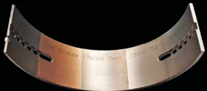
Diagram of bearing shell with layers of composite materials
